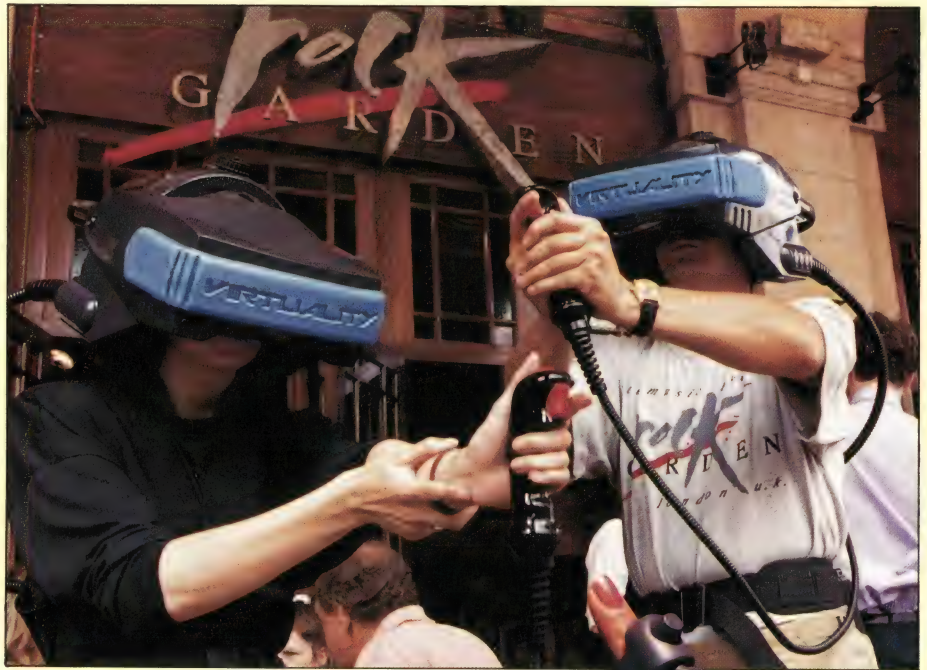
The joystick like hand-held units can be combined with the 'Vissette' for fully mobile interaction in a scanned area.
